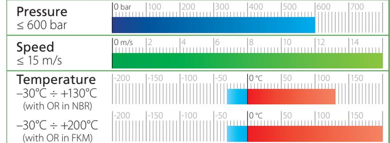
**Fluids** High compatibility with nearly all fluids (with the right choice of O-Ring material)
