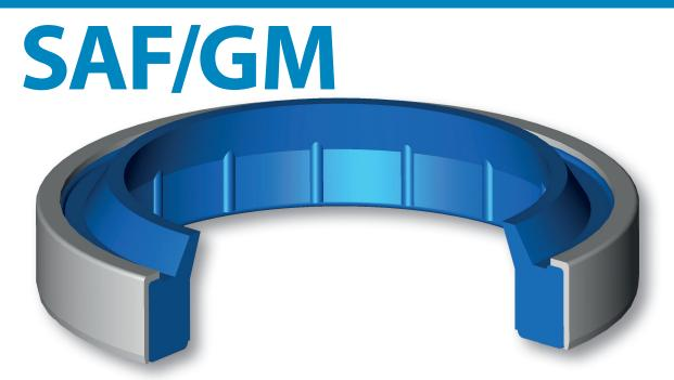
The function of the Aston Seals SAF/GM wiper ring is to prevent introduction of dust, dirt and foreign matter into the system. This is achieved by a special wiper lip which produces a very effective cleaning action, prevents the development of scores, protects the guiding parts and extends the service life of the axial moving rod seals.
