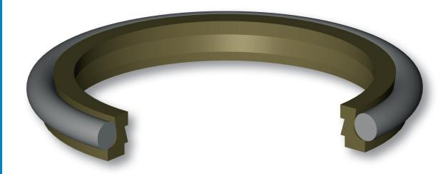
The function of the Aston Seals S2A wiper ring is to prevent introduction of dust, dirt and foreign matter into the system. This wiper can carry out good sealing action if used in conjunction with a rod seal with hydrodynamic back-pumping function. It is composed of:
