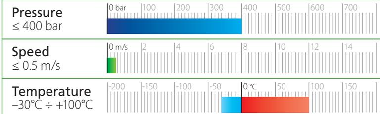
**Fluids** Hydraulic oils (mineral oil based)
